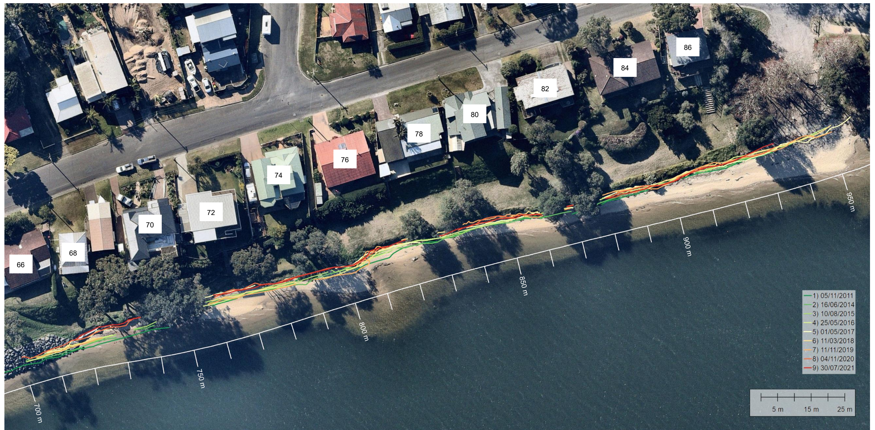
Figure 4.8 Mapping of the position of the bank toe at the back of the beach (2011 to 2021) (Background Image, Nearmap 30/07/2021)
