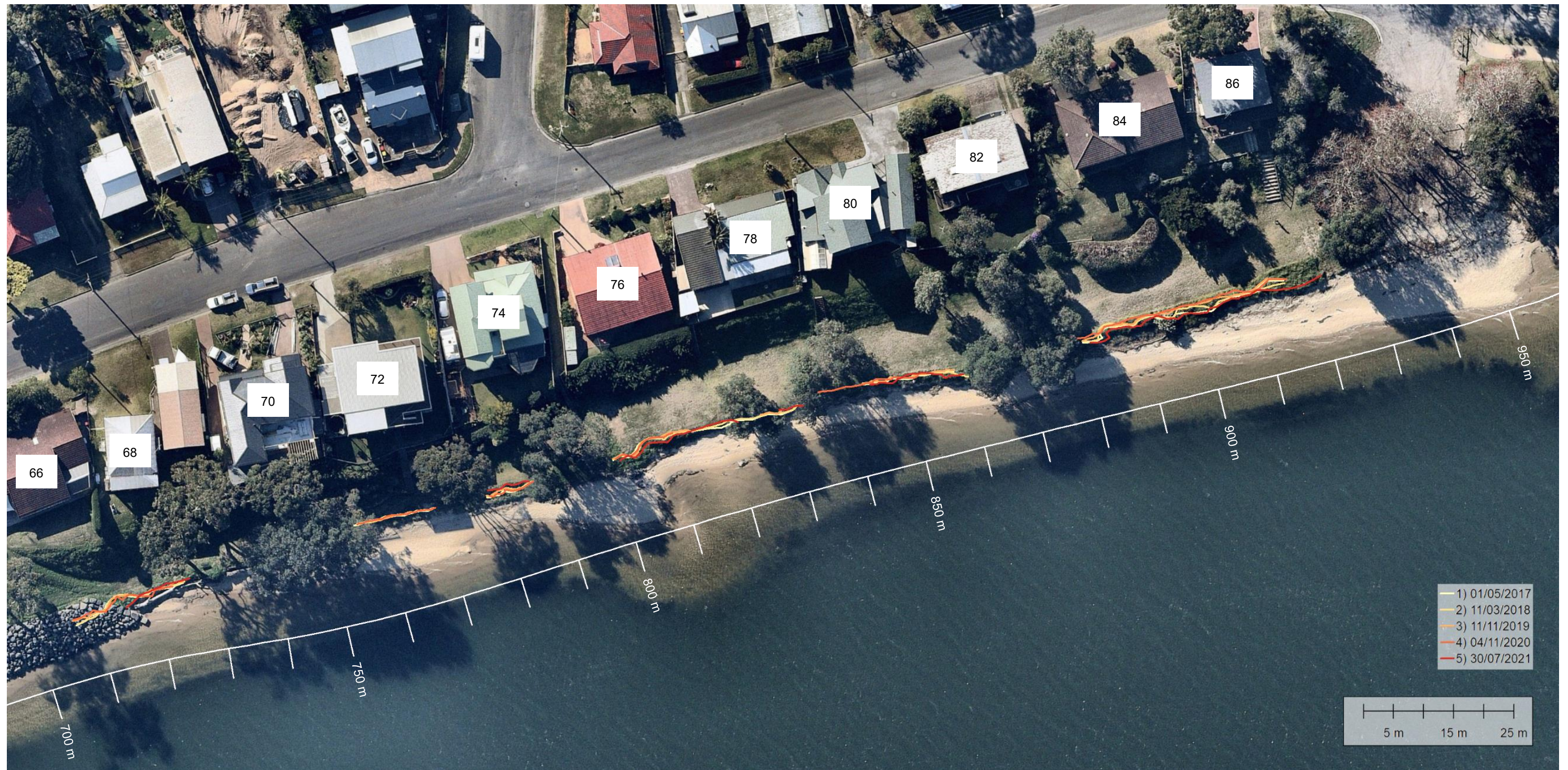
Figure 4.12 Mapping of the position of the bank top at the back of the beach (2017 to 2021) (Background Image, Nearmap 30/07/2021)
