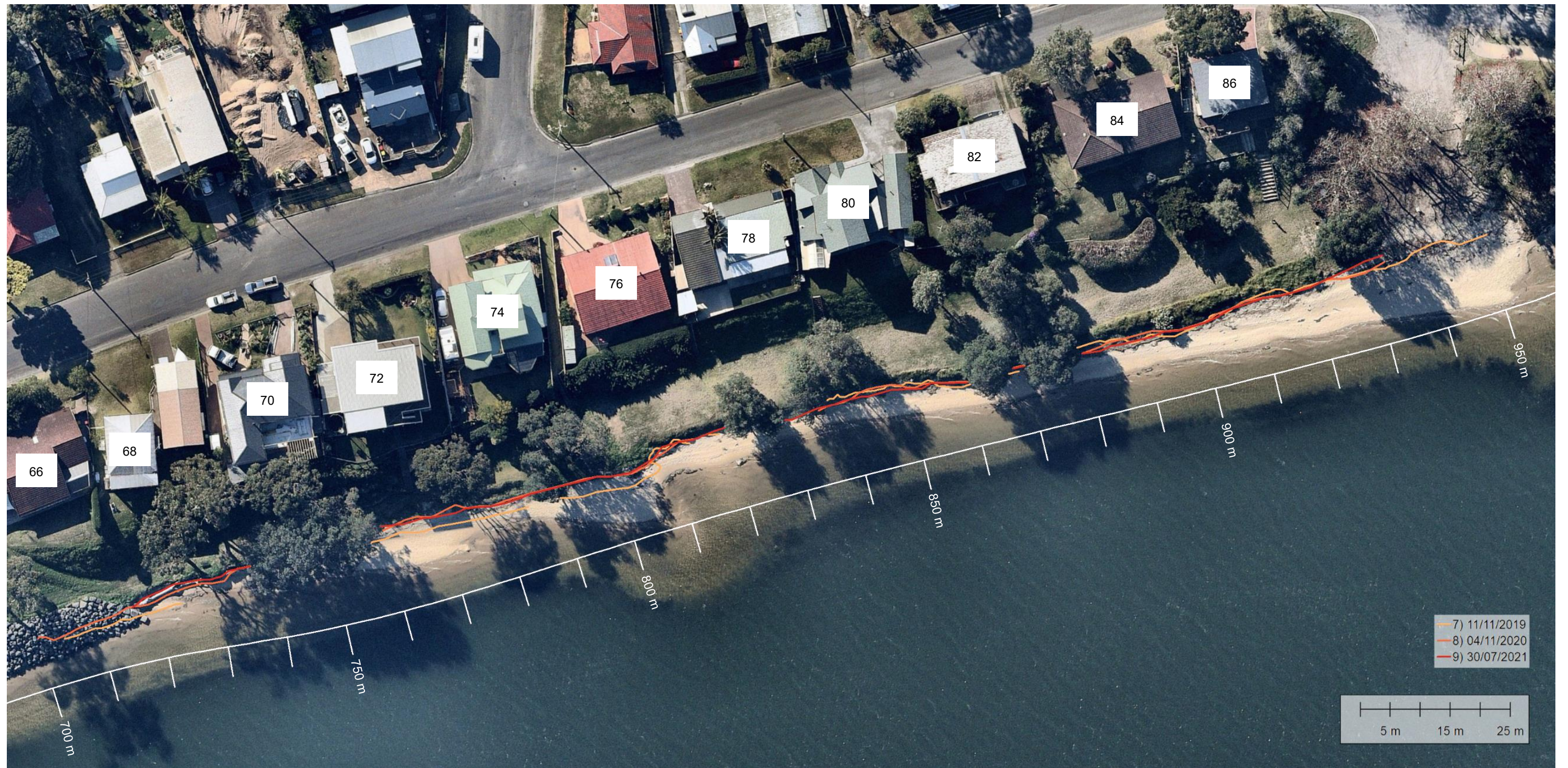
Figure 4.11 Mapping of the recent position of the bank toe between 2019 and 2021 (Background Image, Nearmap 30/07/2021)
