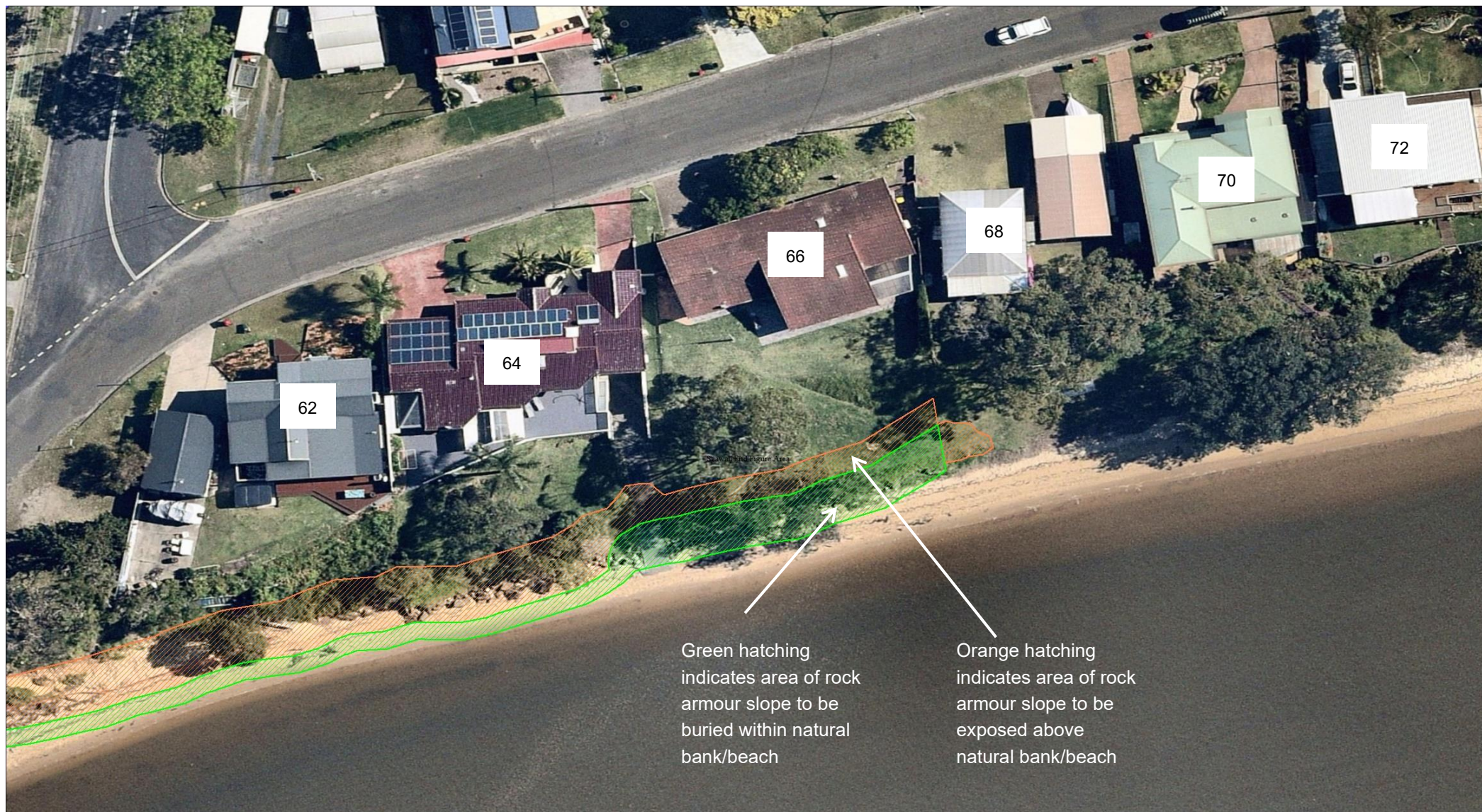
Figure 3.10 Magryn design revetment alignment, pre-construction background image (Image: Nearmap 4/11/2020)
