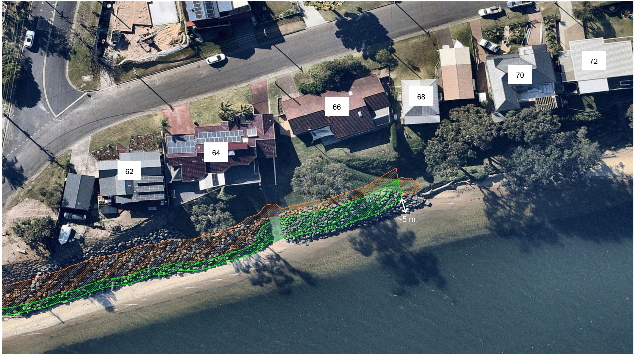
Figure 3.11 Magryn design revetment alignment, post-construction background image (Image: Nearmap 30/07/2021)
