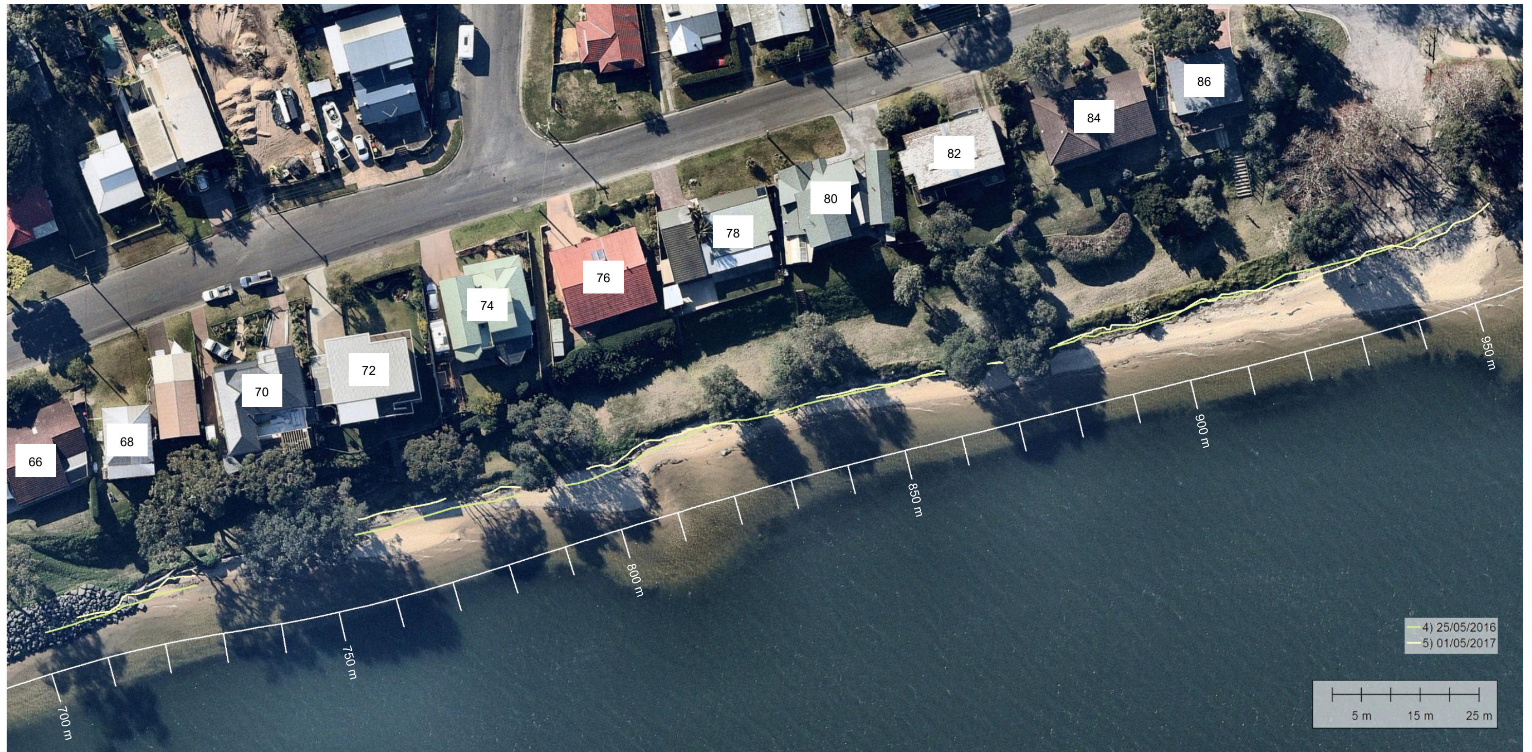
Figure 4.9 Mapping of the position of the bank toe before and after 2016 storms (Background Image, Nearmap 30/07/2021)
